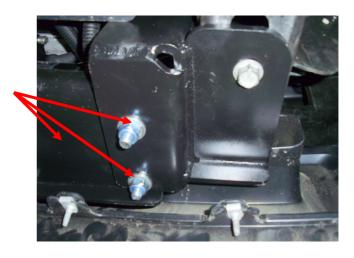
17. The remote control socket position - connect plate No. 4, from the inside of the grill.
