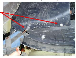
5.Openthe two screws on both sides of the vehicle, located under the bumper.
