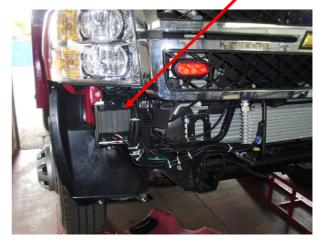
7.Please move the "+" cable that comes out of the control box and goes under the right headlight, goes towards the battery on the right side and connects to the "+" of the circuit breaker.
