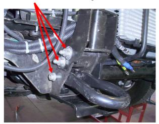
14. Strengthen the bracket by inserting the original fourth screw and closing it with an original nut.
