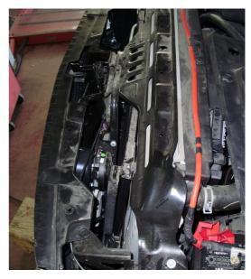
4.Remove the two screws located between the radiator and the grill as shown in the picture (on the left + right side).
