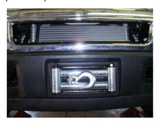
15. After connecting the brackets, install the winch bracket (No. CHW08.030.000) with the help of the four screws (No. 13 in the drawing).
