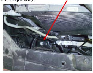
6.Before placing the control box, remove the original bumper. The location of the control box is on the right side of the vehicle under the right headlight.
