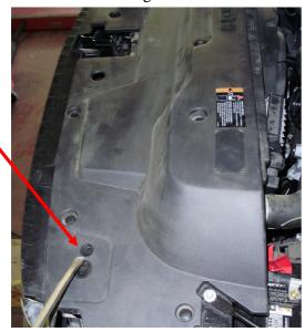
3.Remove the two screws (right side + left side) under the original bumper.
